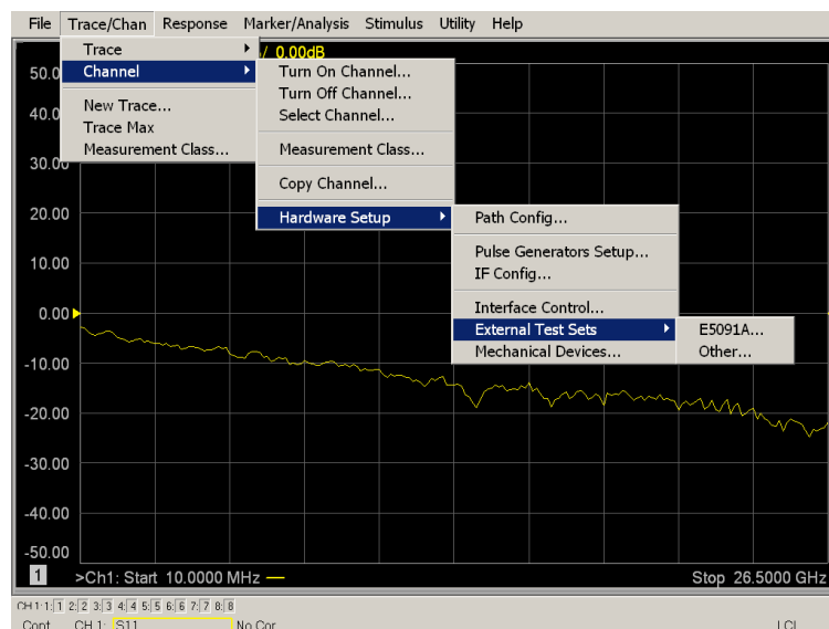
Figure 20 External Test Set Control
